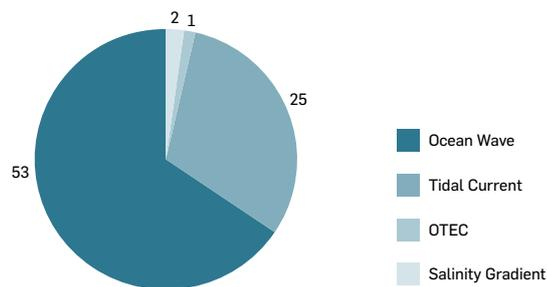
This study has identified 81 individual concepts currently in development<sup>5</sup>. These include: 53 reported ocean wave technologies in development; 25 tidal current projects; one OTEC system and two salinity gradient concepts (see Figure 2.1). The current number of ocean wave technologies in
