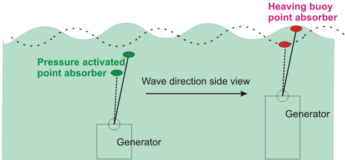
Figure 1: Pressure activated and heaving buoy point absorbers
